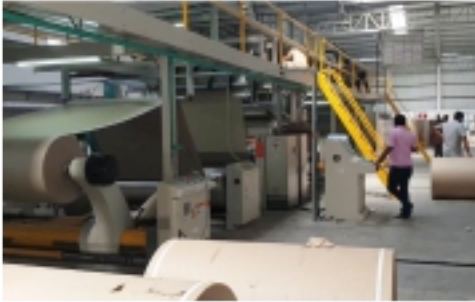
Automatic Corrugated Board Making Plant
