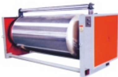
Pre Heater / Conditioner
